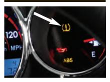
The Tire Pressure Monitor alerts you when a significant reduction in pressure occurs in one or more of your vehicle's tires by illuminating the  $\langle \underline{l} \rangle$  (Low Tire Pressure) warning light on the instrument panel. The low tire pressure warning light will remain on until you correct the tire pressure.
