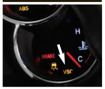
StabiliTrak is a Vehicle Stability Control (VSC) system that uses an advanced computer to assist your vehicle with directional control during difficult driving situations.
