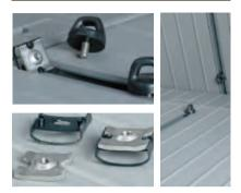
At vehicle delivery, cargo tie-downs and a corresponding installation diagram were provided under the rear cargo floor panel.
