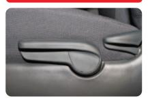
To adjust the driver's seat height, pull the lever located on the outboard side of the seat cushion until reaching the desired height. (You may find the seat easier to adjust when unoccupied.) Before adjusting, make sure the ignition is off and the vehicle is in Park (P).
