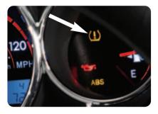
The Tire Pressure Monitor alerts you when a significant reduction in pressure occurs in one or more of your vehicle's tires by illuminating the <!>) (low tire pressure) warning light on the instrument panel. The low tire pressure warning light will remain on until you correct the tire pressure.
