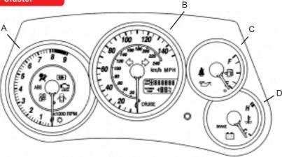
Your vehicle's instrument panel is equipped with this cluster or one very similar to it. The instrument panel cluster includes these key features:
