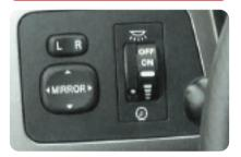
The dome lamp control dial is located on the instrument panel to the left of the steering wheel. To operate the lamp, follow these instructions:
