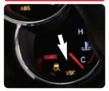
This Vehicle Stability Control (VSC) system uses an advanced computer to assist your vehicle with directional control during difficult driving situations.
