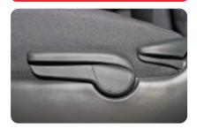
To adjust the driver's seat height, pull the lever located on the outboard side of the seat cushion until reaching the desired height. (You may find the seat easier to adjust when unoccupied.) Before adjusting, make sure the ignition is off and the vehicle is in Park (P).
