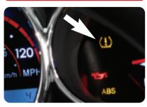
The system alerts you when it detects a large change in the pressure of one tire. The system cannot alert you before you drive that a tire is low or flat. The Tire Pressure Monitor System does not replace normal tire maintenance.
