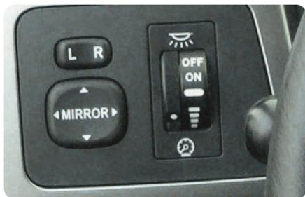
The interior dome lamp control dial is located on the instrument panel to the left of the steering wheel. To operate the lamp, follow these instructions:
