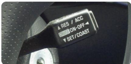
The cruise control lever is located on the right side of the steering wheel. Cruise Control operates only at speeds above 25 mph. When vehicle speed drops below this point, Cruise Control turns off and the system erases the set speed.
