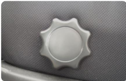
To adjust the height of the driver's seat, turn the knob located on the outboard side of the driver's seat cushion. It is easier to adjust when the seat is unoccupied. Make sure the ignition is off and the vehicle is in PARK (P) before adjusting the seat.
