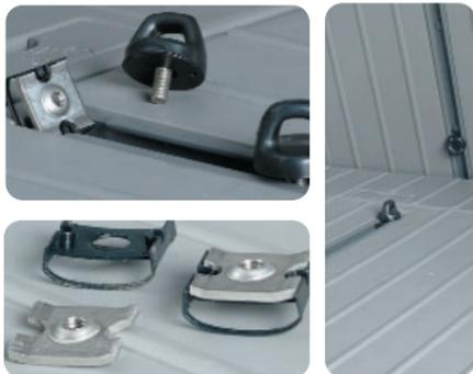
At vehicle delivery, four cargo tie-downs with a corresponding installation diagram were provided under the rear cargo floor panel.
