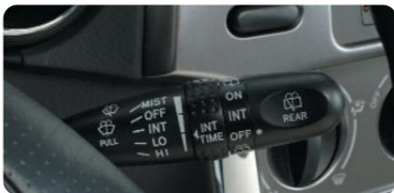
To reduce the possibility of scratched rear liftglass, activate the washer prior to the wipers by rotating the rear wiper switch downward. After pre-washing the rear liftglass, rotate the switch to the upper washer position to activate the washer and the rear wiper together.
